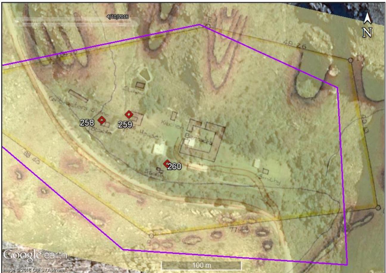
Figure 40: Composite image created by superimposing Survey Diagram 667/1872 onto the modern aerial view. The purple polygon is, according to Cape Farm Mapper, the correct farm boundary.
